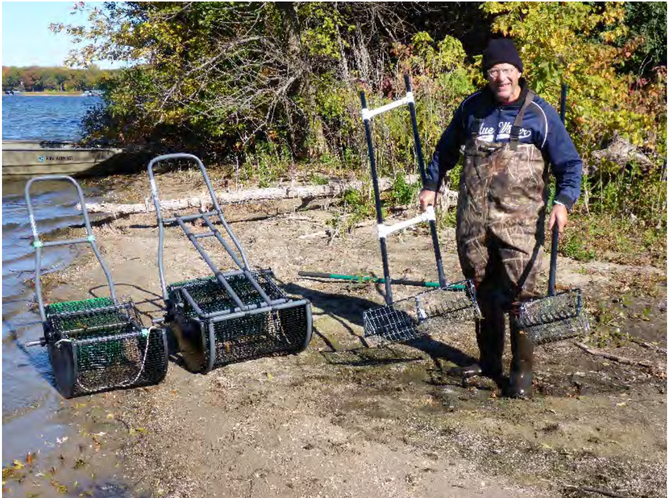
Figure S2. Zebra mussel collection devices for small-scale removal projects. These devices can be used to pick up clumps of zebra mussels.
