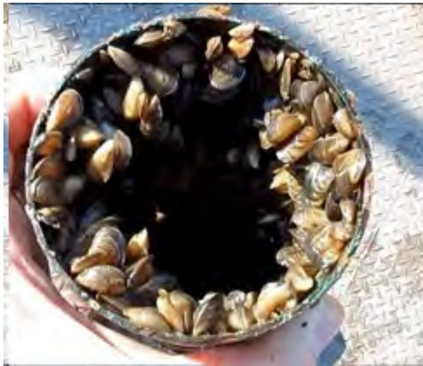
Zebra mussels will attach and grow in large and small diameter pipes and water lines.
